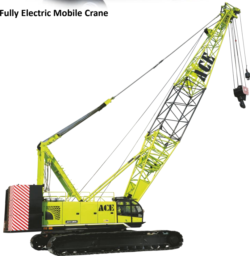
180 Tons Crawler Crane
